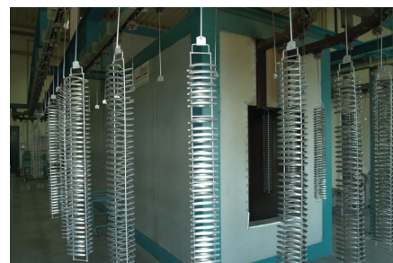
Schwinn's fully automated, high volume powder coating machine.
